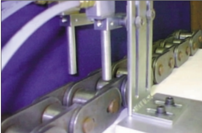
Roller chain with spray nozzle
